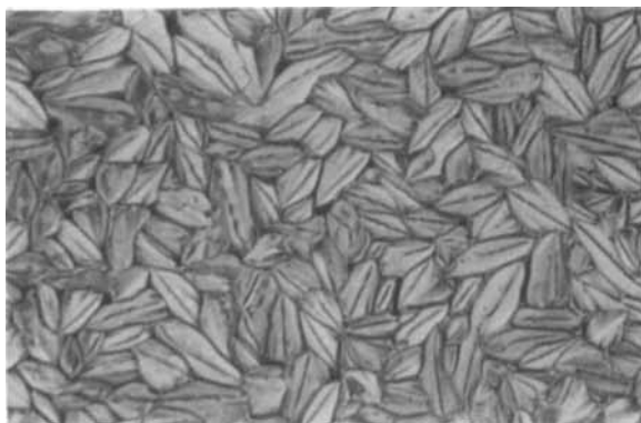
FIGURE 1 Smectic C^* phase of compound 7b in the polarizing microscope (214 °C) (See color plate XIX at the back of this issue)
